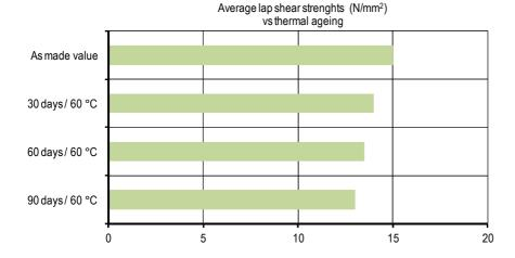
The tests have been carried out at 20 °C on steel to steel joints, which have been aged at 60 °C. At the end of the 3 thermo cycles of 24 hours each ranging from -40 °C to 100 °C, there has been no variation in the average lap shear strength. Pre-treatment has been made by sanding and degreasing with acetone.
