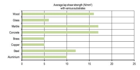
The tests have been conducted at 20°C on metal to metal joints, which have been hardened for 48 hours at 20°C.
